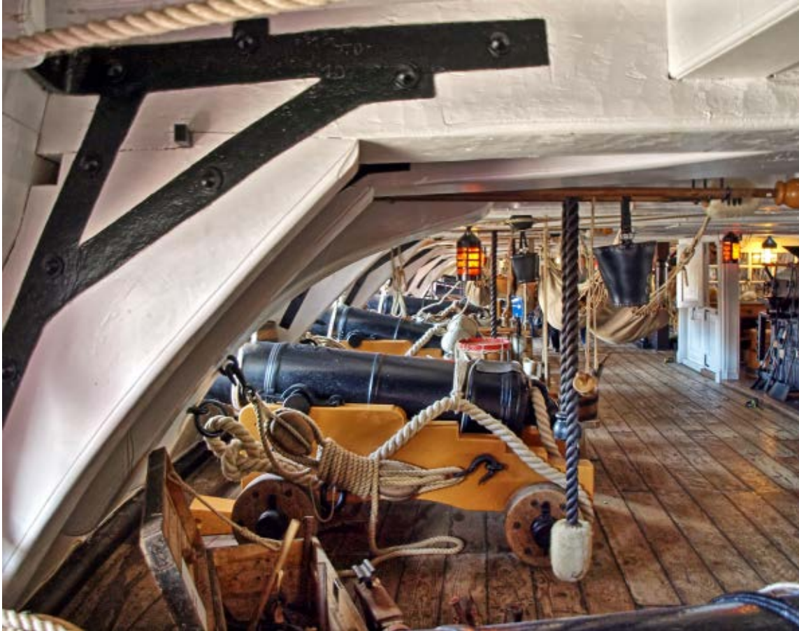
Photograph of the lower gun deck showing a chock, with the Roberts plate in position. Courtesy of Neil Howard Photos
